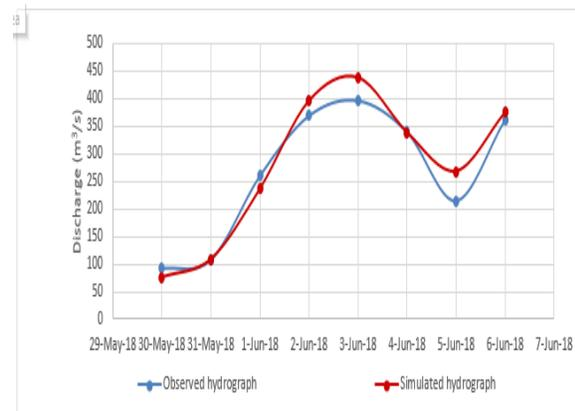
Figure 8: Observed and simulated hydrographs for Validation event 1- Combination 3
