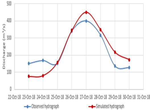
Figure 9: Observed and simulated hydrographs for Validation event 2- Combination 3
