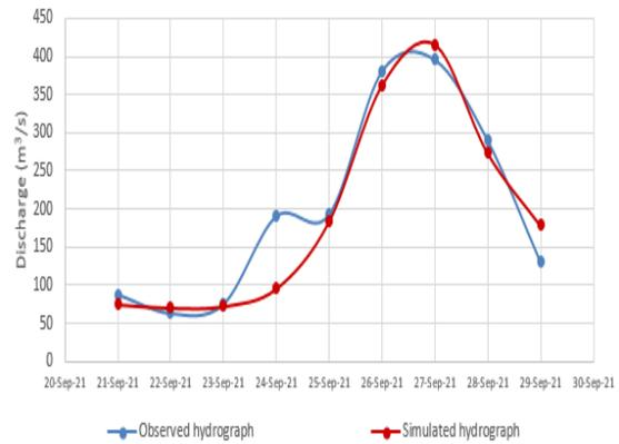
Figure 10: Observed and simulated hydrographs for Validation event 3- Combination 3
